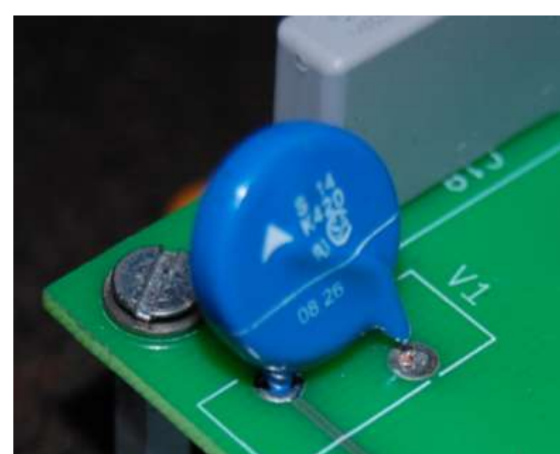
Pin fracture of heavy component
